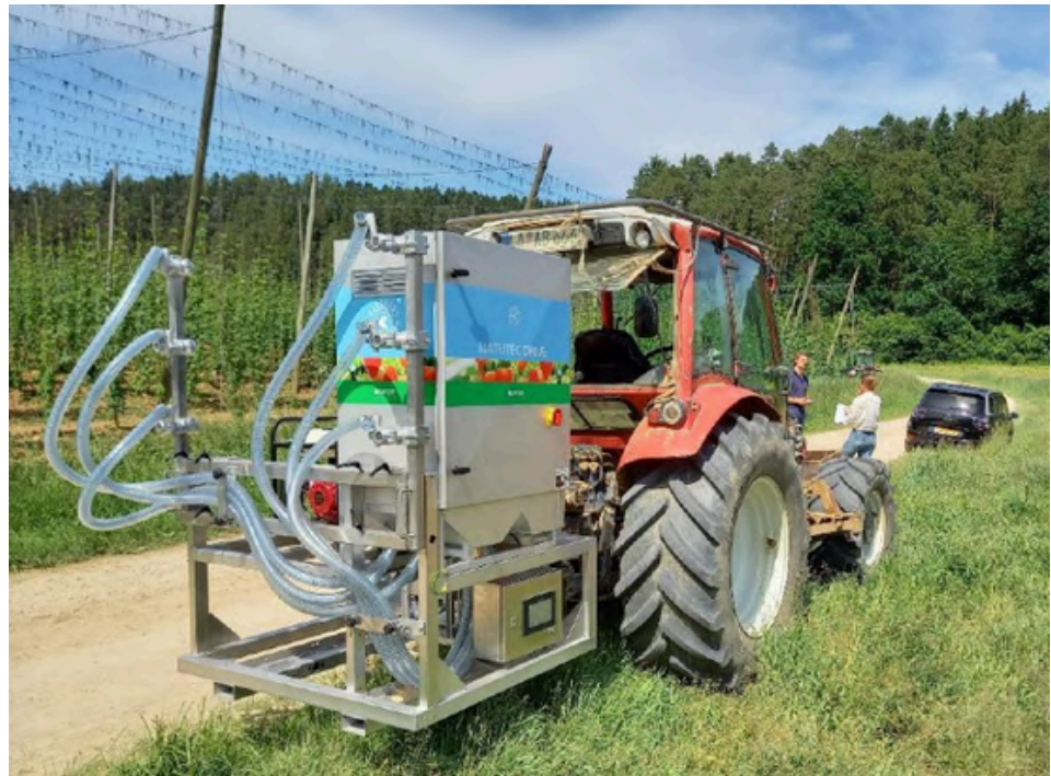
Prototype for mechanical release of predatory mites; (image: meeting documentation by Florian Weihrauch).
